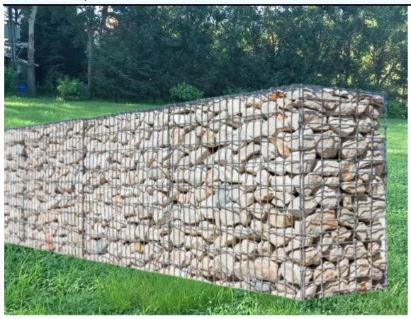
**Welded Gabion Baskets** are made of welded wire nets and filled with stones. Welded gabion nets are made of thicker wires so that the mesh is strong enough and tear-resistant. The wire is covered by zinc or galfan which protects it from the effects of the weather for a long time.
